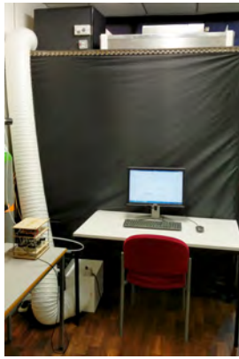
Figure 4. Olfactory interaction space: clean room wrapped into a black water repellent fabric with an air extractor E1 and the clean air blower on the top, as well as a scent-delivery device and an air extractor E2 in the bottom-left corner (outside the clean room).
